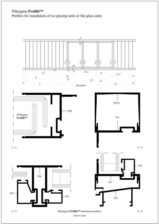
figure 10-25: Profiles for installation of iso glazing units or flat glass units, DXF (25)
