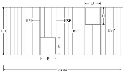
figure 6-5: Schematic view of a Pilkington **Profilit<sup>TM</sup>** facade
