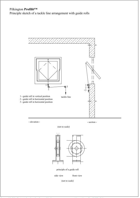
figure 10-21: Principle sketch of a tackle line arrangement with guide rolls, DXF (21)
