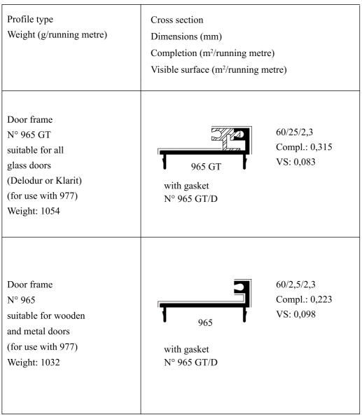
figure 9-16: Aluminium and plastic profiles for Pilkington **Profilit™** glazing (NP/SP), DXF (16)
