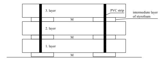
Storage of Profilit<sup>™</sup> profiled glass - side view of stack 2/3 of the storage surface is of styrofoam Leave centre (M) free for lifting equipment
