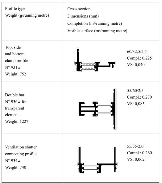
figure 9-19: Aluminium and plastic profiles for Pilkington **Profilit™** glazing (NP/SP), DXF (19)
