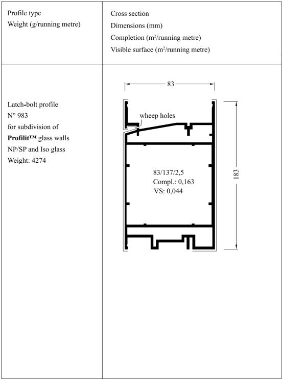
figure 9-7: Aluminium and plastic profiles for Pilkington **Profilit™** glazing (NP/SP), DXF (7)
