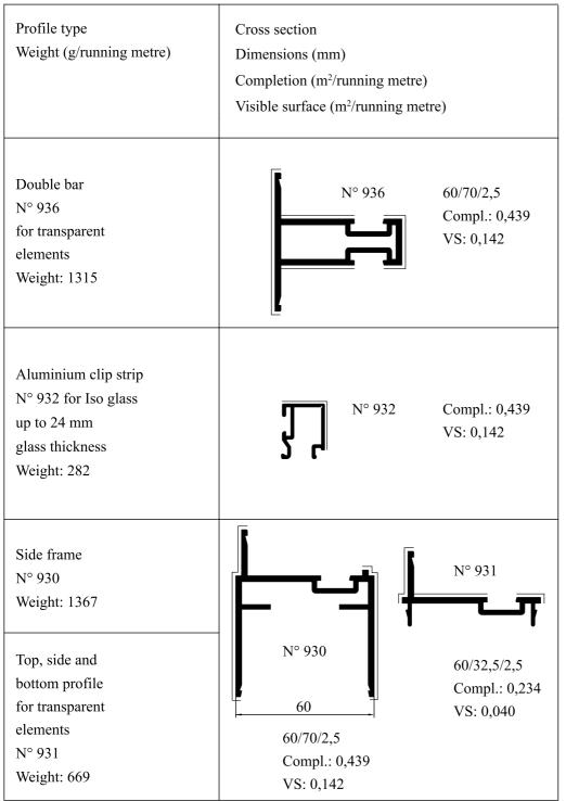
figure 9-17: Aluminium and plastic profiles for Pilkington **Profilit™** glazing (NP/SP), DXF (17)
