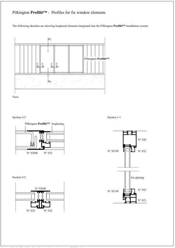
figure 10-6: Profiles for fix window elements, DXF (6)
