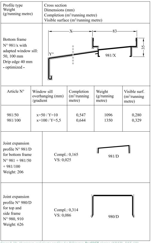
figure 9-10: Aluminium and plastic profiles for Pilkington **Profilit™** glazing (NP/SP), DXF (10)
