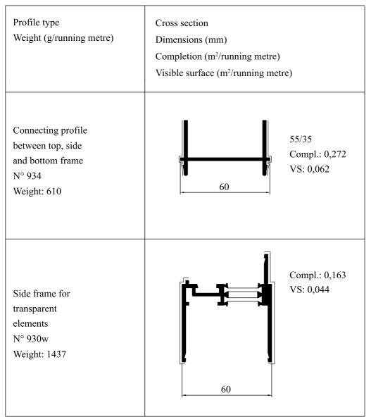
figure 9-18: Aluminium and plastic profiles for Pilkington **Profilit™** glazing (NP/SP), DXF (18)
