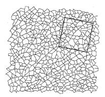
Figure 1: Select the area of coarsest fracture, place the template on the test specimen and draw round the template.
