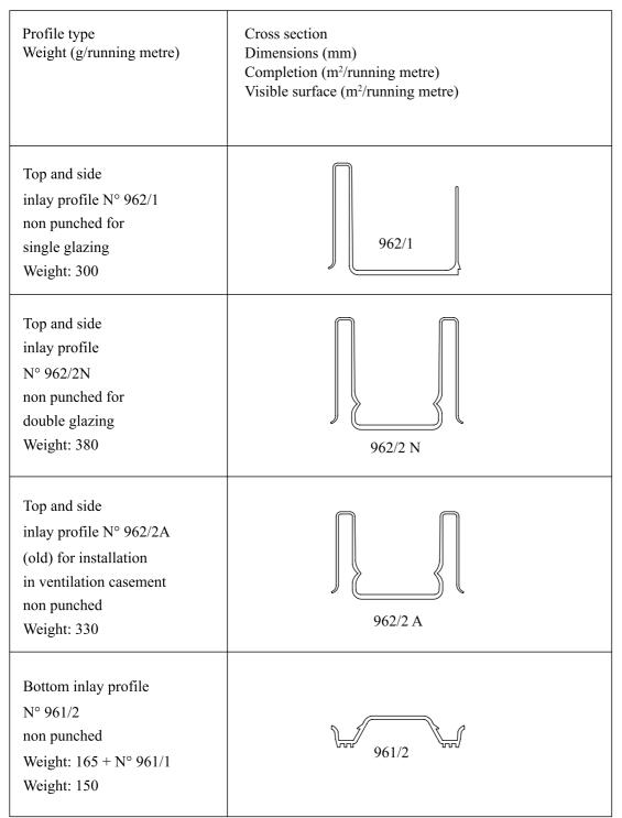
figure 9-3: Aluminium and plastic profiles for Pilkington **Profilit™** glazing (NP/SP), DXF (3)
