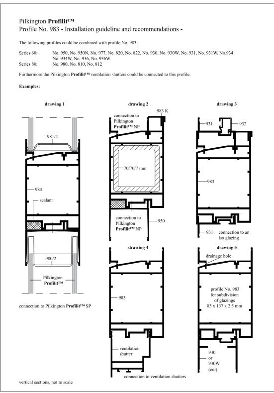
figure 10-30: Profile No. 983 - Installation guideline and recommendations -, DXF (30)
