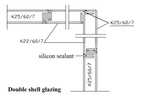
at least one glass run must be cut lengthwise and pad by profile N° 166
