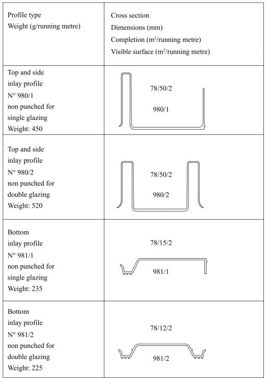
figure 9-20: Aluminium and plastic profiles for Pilkington **Profilit<sup>TM</sup>** glazing (NP/SP), DXF (20)
