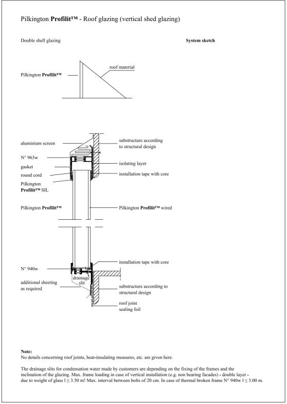
figure 10-5: Roof glazing (vertical shed glazing), DXF (5)
