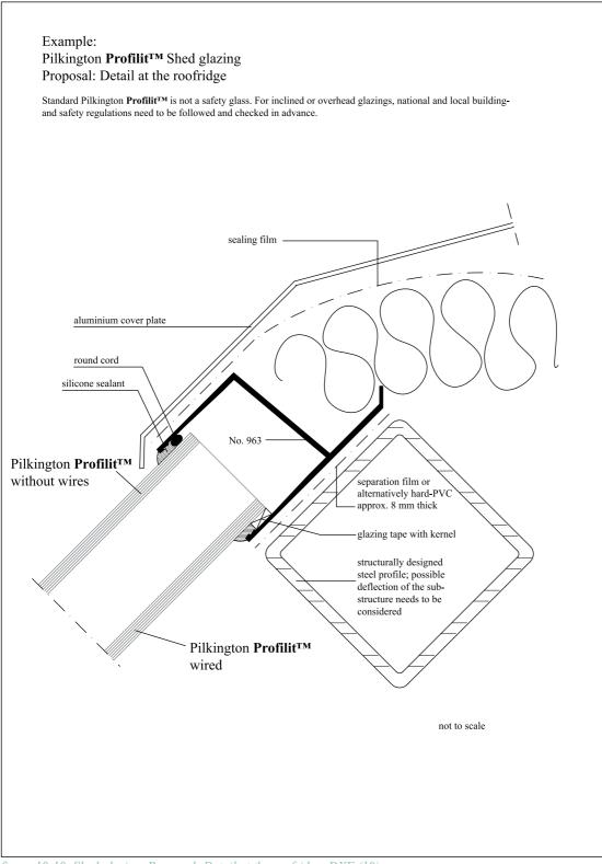
figure 10-10: Shed glazing, Proposal: Detail at the roofridge, DXF (10)
