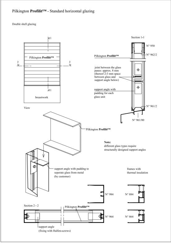
figure 10-3: Standard horizontal glazing, DXF (3)
