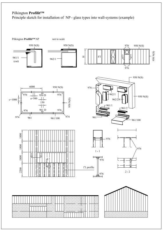
figure 10-23: Principle sketch for installation NP glass types into wall-systems (example), DXF (23)
