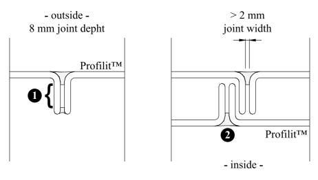
figure 8-3: Sealing profiled glass runs with Pilkington **Profilit<sup>IM</sup>** SIL, sketch (not to scale)
