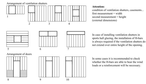
figure 8-6: Installation of ventilation shutters
