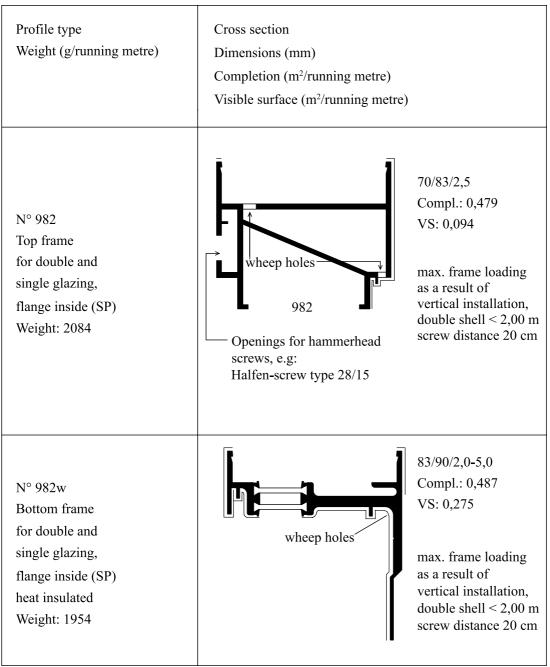
figure 9-15: Aluminium and plastic profiles for Pilkington **Profilit™** glazing (NP/SP), DXF (15)
