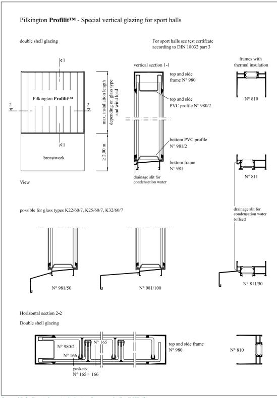
figure 10-2: Special vertical glazing for sport halls, DXF (2)
