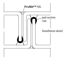
figure 8-2: Arrangement of pad section N° 166 for roof glazing
