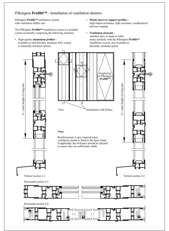
figure 10-7: Installlation of ventilation shutters, DXF (7)
