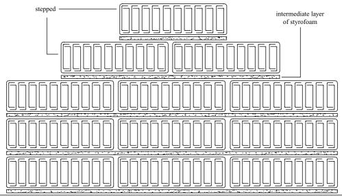
figure 2-1: Storage of Pilkington **Profilit<sup>TM</sup>** profiled glass for building – side view of stack
