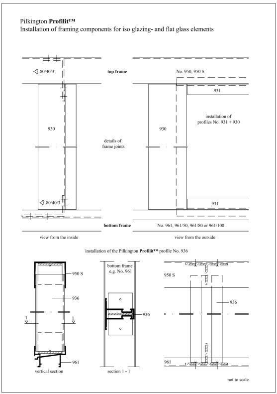
figure 10-26: Installation of framing components for iso glazing- and flat glass elements, DXF (26)
