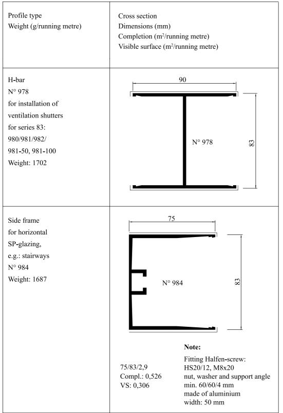
figure 9-11: Aluminium and plastic profiles for Pilkington **Profilit<sup>TM</sup>** glazing (NP/SP), DXF (11)
