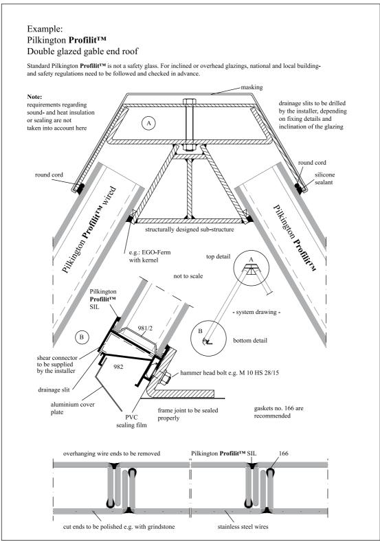
figure 10-11: Double glazed gable end roof, DXF (11)
