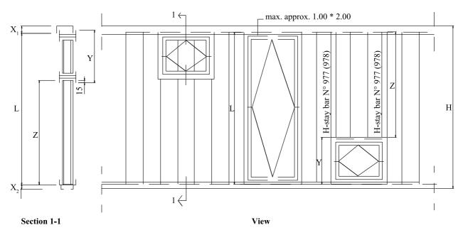
figure 7-3: Glass length over or under the ventilation element, sketch
