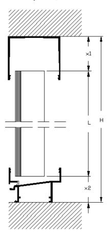
figure 7-1: Calculation of glass length
