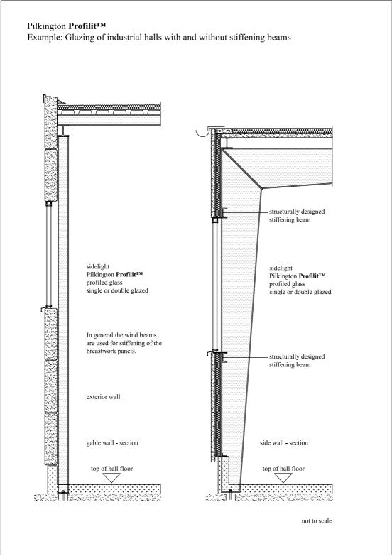
figure 10-24: Example: Glazing of industrial halls with and without stiffening beams, DXF (24)
