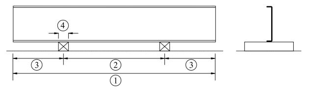
figure 11-3: Measurement of overall bow
