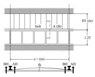
figure 6-9: Pilkington **Profilit<sup>TM</sup>** profiled glass window runs over visual fixed window elements
