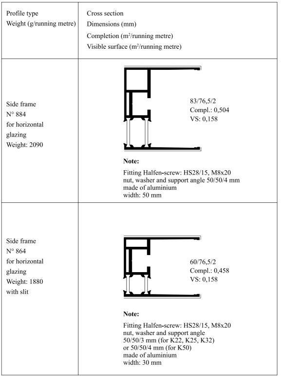
figure 9-27: Aluminium and plastic profiles for Pilkington **Profilit™** glazing (NP/SP), DXF (27)
