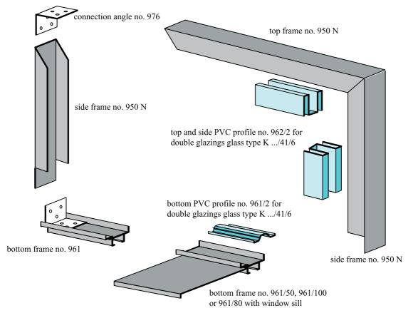
figure 2-4: Pilkington **Profilit<sup>TM</sup>** framing system (e.g. NP-series 60)
