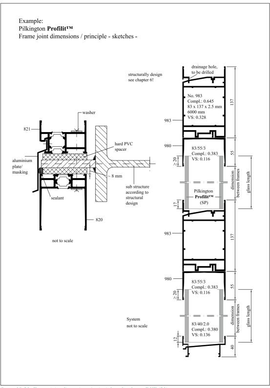
figure 10-31: Frame joint dimensions / principle - sketches -, DXF (31)
