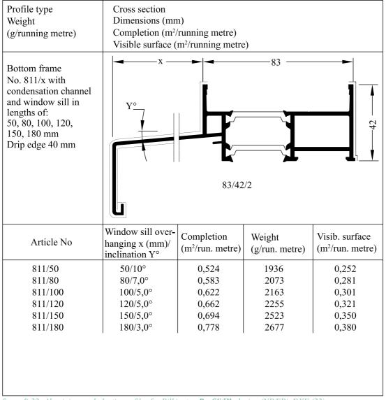
figure 9-22: Aluminium and plastic profiles for Pilkington **Profilit<sup>TM</sup>** glazing (NP/SP), DXF (22)
