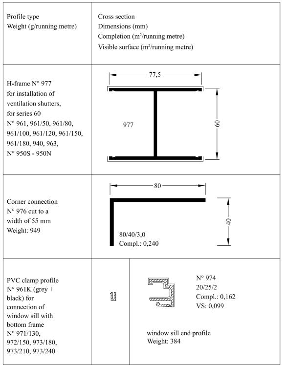
figure 9-6: Aluminium and plastic profiles for Pilkington **Profilit<sup>™</sup>** glazing (NP/SP), DXF (6)
