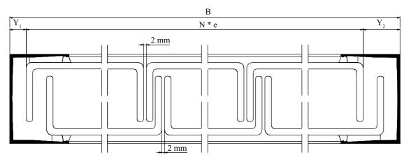
Horizontal section - double shell glazing (N = number of glass panes, e = centreline dimension acc. to 7.2.5.)
