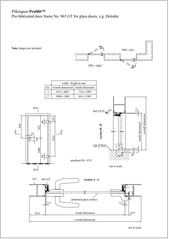
figure 10-28: Pre-fabricated door frame No. 965 GT for glass doors, e.g. Delodur, DXF (28)
