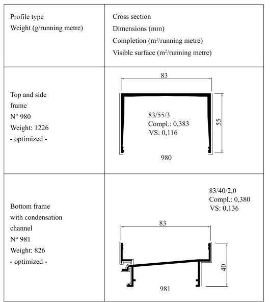
figure 9-9: Aluminium and plastic profiles for Pilkington **Profilit<sup>TM</sup>** glazing (NP/SP), DXF (9)
