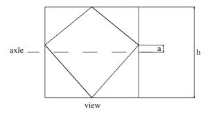
figure 8-9: Off-centre bearing of Pilkington Profilit™ pivoting lights
