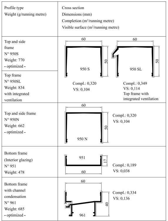
figure 9-2: Aluminium and plastic profiles for Pilkington **Profilit<sup>TM</sup>** glazing (NP/SP), DXF (2)
