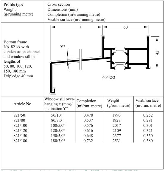
figure 9-25: Aluminium and plastic profiles for Pilkington **Profilit<sup>TM</sup>** glazing (NP/SP), DXF (25)
