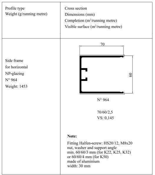
figure 9-8: Aluminium and plastic profiles for Pilkington **Profilit™** glazing (NP/SP), DXF (8)
