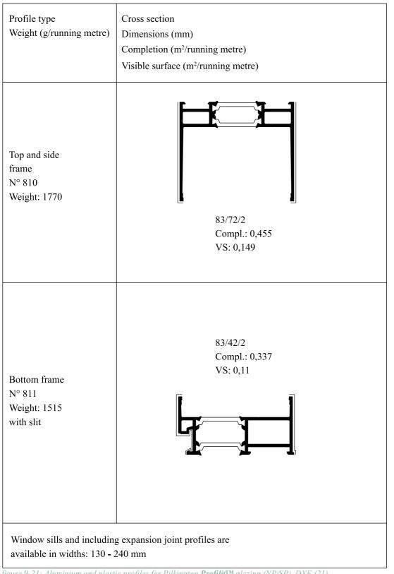
figure 9-21: Aluminium and plastic profiles for Pilkington **Profilit™** glazing (NP/SP), DXF (21)
