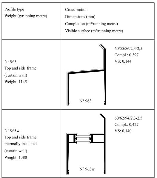
figure 9-14: Aluminium and plastic profiles for Pilkington **Profilit™** glazing (NP/SP), DXF (14)
