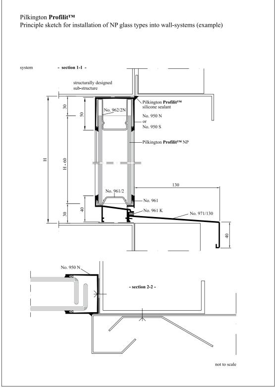
figure 10-22: Principle sketch for installation of NP glass types into wall-systems (example), DXF (22)
