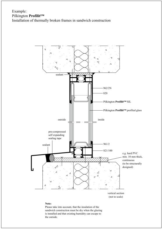
figure 10-29: Installation of thermally broken frames in sandwich construction, DXF (29)
