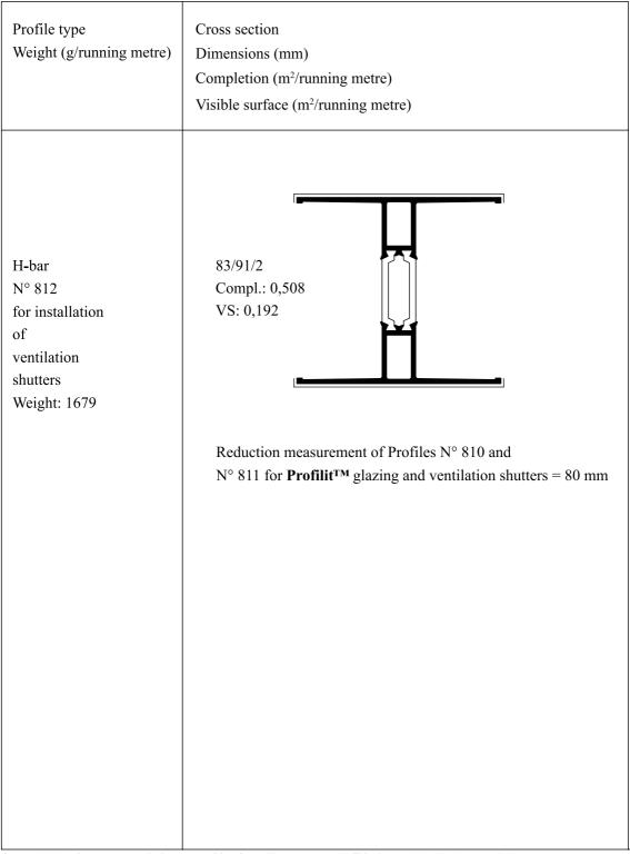
figure 9-23: Aluminium and plastic profiles for Pilkington **Profilit<sup>TM</sup>** glazing (NP/SP), DXF (23)
