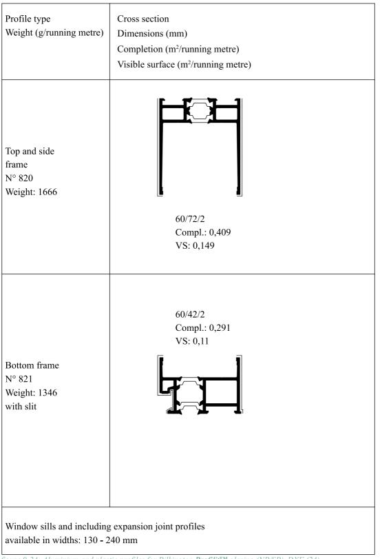
figure 9-24: Aluminium and plastic profiles for Pilkington **Profilit<sup>TM</sup>** glazing (NP/SP), DXF (24)
