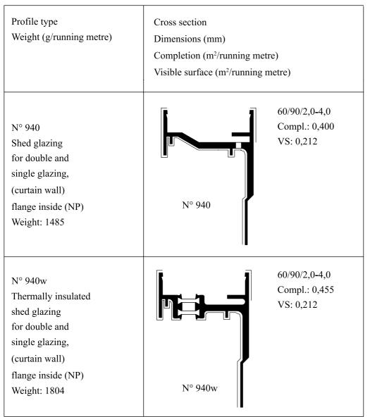
figure 9-13: Aluminium and plastic profiles for Pilkington **Profilit<sup>TM</sup>** glazing (NP/SP), DXF (13)
