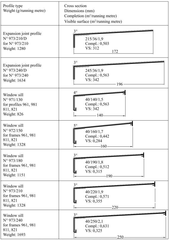
figure 9-5: Aluminium and plastic profiles for Pilkington **Profilit<sup>TM</sup>** glazing (NP/SP), DXF (5)
