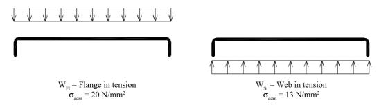
figure 6-2: Application of section modulus
