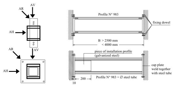
The number, type, size and spacing of the fixing dowels should be determined on the basis of local conditions.
