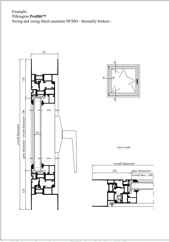
figure 10-20: Swing and swing tilted casement SP/ISO - thermally broken -, DXF (20)
